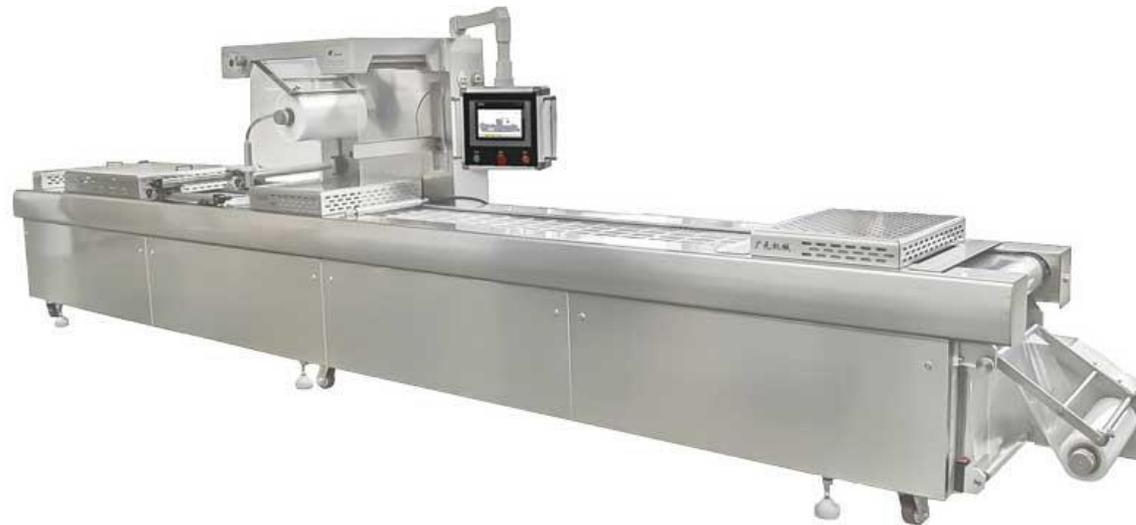
Rollstock/Thermoforming vacuum packaging machine, fully customized according to package size and product characteristics. Possibility to package different sizes and different products in 1 machine.
