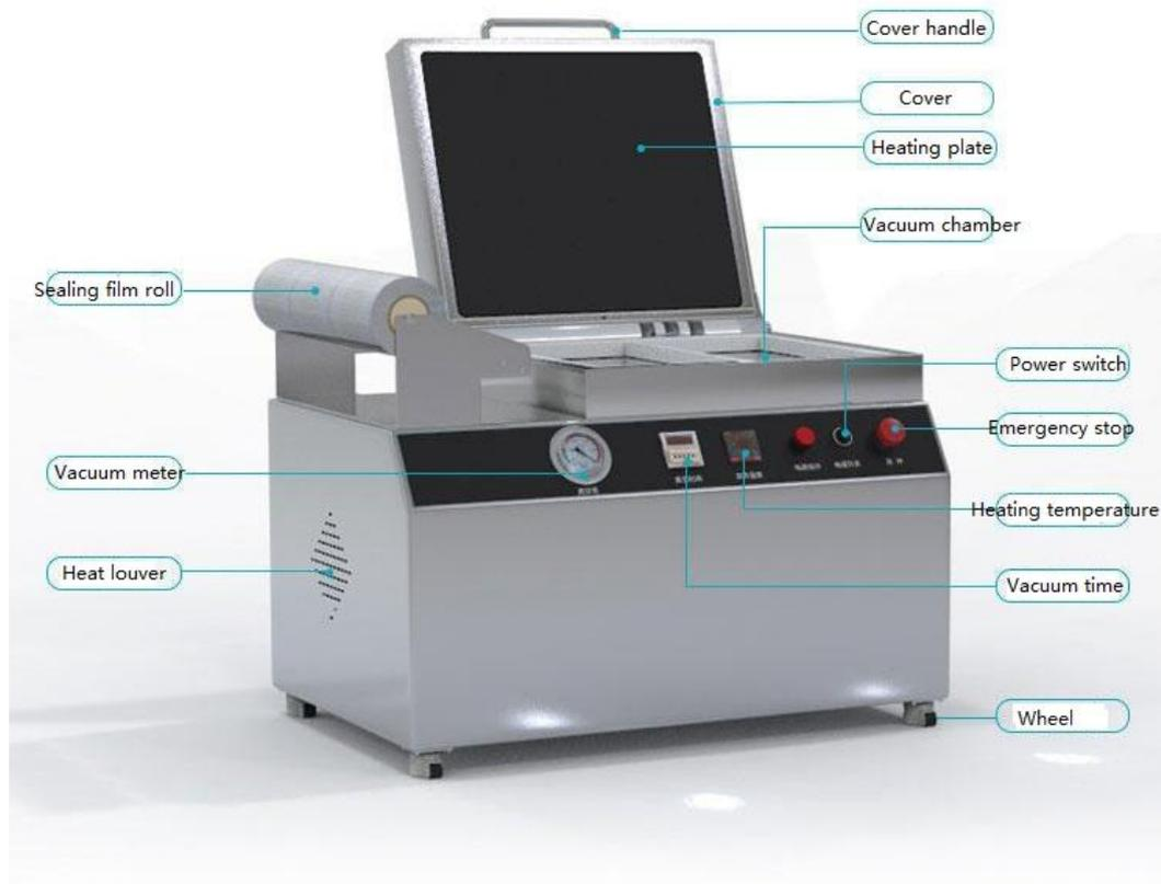
Tabletop vacuum skin packaging machine is mainly composed of vacuum chamber, heating plate, SUS304 machine frame, vacuum system, electric control system.
