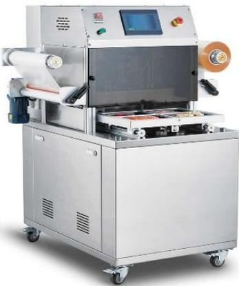
A vertical skin pack machine with a stainless steel cabinet on wheels. It has a control panel on the top front. A roll of packaging material is being processed, and a finished package is visible on the right side.                                                       |                                               |                                                 |                                                               |
